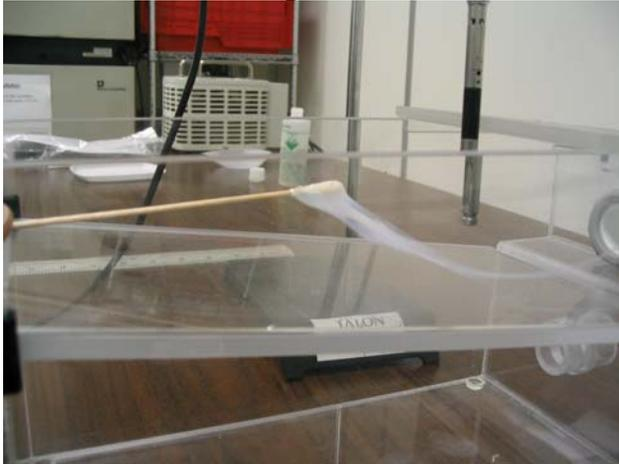
Elevation of 2-Liter Chamber Showing Airflow Capture (note anemometer in slot test-pos.)
