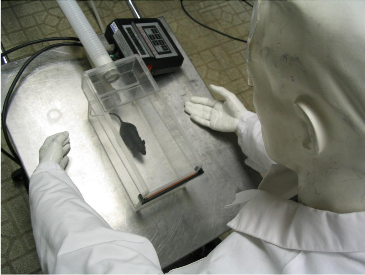
Tracer Gas Test Geometry (~14" viewing distance to top of 'Chamber; Simulated Rodent)
