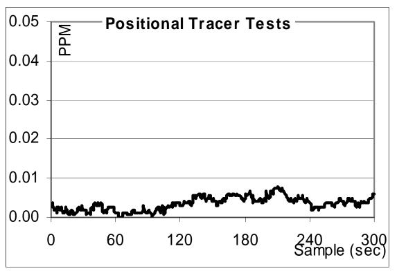
Diagram 5: Tracer Gas Test Plot: -0.50" wc Static Pressure
