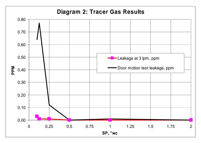
(The data suggests that the COMPAC5 begins to lose its ability to capture below 0.125"wc. At no time during our tests did the average Leakage (red trace above) exceed 0.10ppm)
