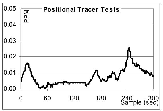
Diagram 6: Tracer Gas Test Plot: -0.25" wc Static Pressure
