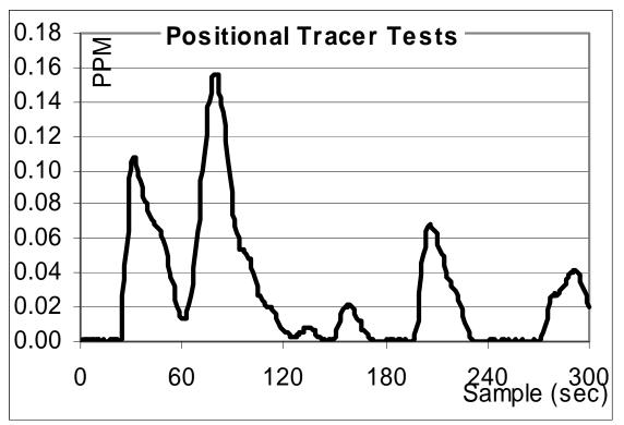
Diagram 8: Tracer Gas Test Plot: -0.10" wc Static Pressure
