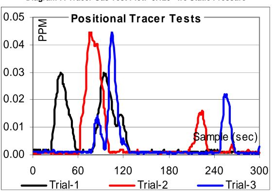
Diagram 7: Tracer Gas Test Plot: -0.125" wc Static Pressure
