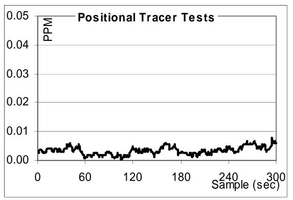
Diagram 3: Tracer Gas Test Plot: -2.00" wc Static Pressure
