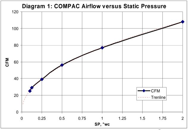
(SP = static pressure, or vacuum at the outlet collar of the  $COMPAC^{5}$ )
