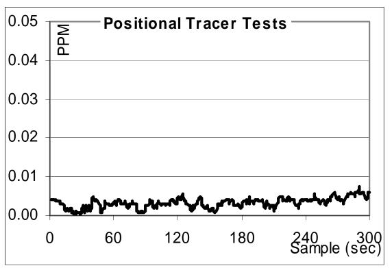
Diagram 4: Tracer Gas Test Plot: -1.00" wc Static Pressure
